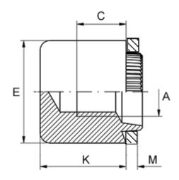
Female thread A = M4Height K = 9.0Min thread length C = 4.0Outer diameter E = 10.0Plate thickness = 2.3 to 2.5
